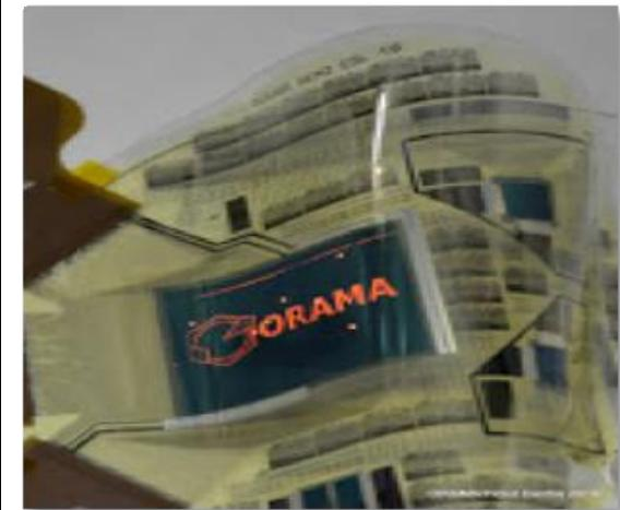
**Flexible OLED Display based on IGZO TFTs, 2014**
